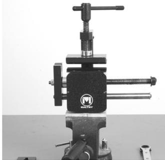
**1.** To set up extractor for use, secure in a vise (as shown).
