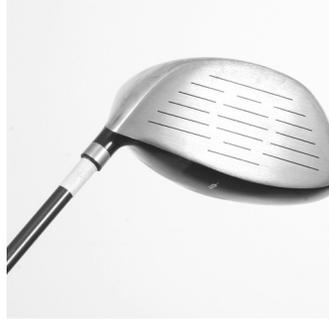
**2.** Remove the ferrule and wrap a 3/4" piece of masking tape around the shaft next to the hosel (as shown). Ferrules can be easily removed by slightly heating with a heat gun to soften, then carefully cut the ferrule off the shaft. Be careful not to cut into the shaft or scratch the head finish.
