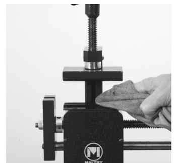
**8.** Keeping the pads and the clamp area clean is critical to how this machine will perform. Use alcohol, acetone or naphtha to clean these surfaces. A clean, tacky pad surface is essential to the shaft staying secure in the vise during the extracting operation.
