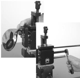
**5.** Place the steel adaptor plate over the shaft between the hosel and the main push block. Make sure it is snug between the pull bar and the hosel. Using the ratchet provided, tighten the large hex head bolt until the main push block is snug against the steel adaptor plate and hosel.
