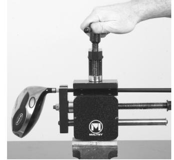
**4.** Place the top clamp piece over the shaft. Tighten top clamping handle until snug. **CAUTION: Over tightening can damage the shaft.**
