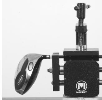
**3.** Before placing the club into the extractor, be sure the main pulling block is as close to the base or center of the puller as possible. Place the club into the extractor, making sure there is 1/2" distance between the top of the hosel and the main push block. This allows ample space to place the steel adaptor plate.
